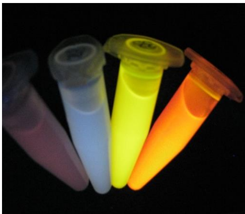
Suspensions of dye-labeled SiO 2 nano-particles under excitation with UV lamp ( \lambda = 365 nm)
